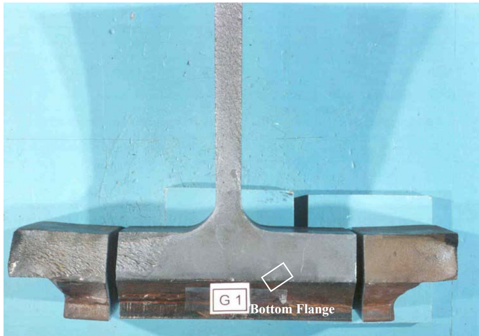
Fig. 8. Exposed Crack Surface at Toe of Cover Plate End Weld
