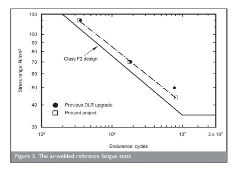
Fatigue strengthening of welds in light rail structures
