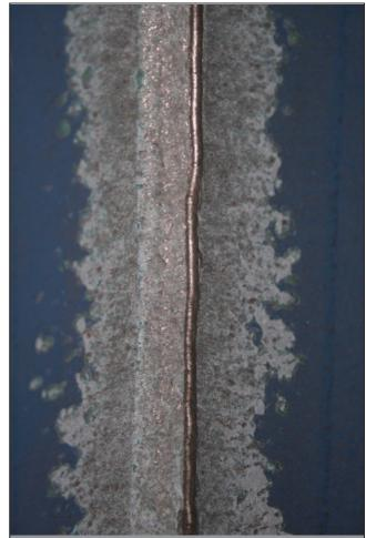
Figure 10. Example of UIT groove
