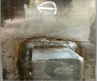
Figure 5. Fatigue crack from weld toe and into main plate of an as-welded test piece
