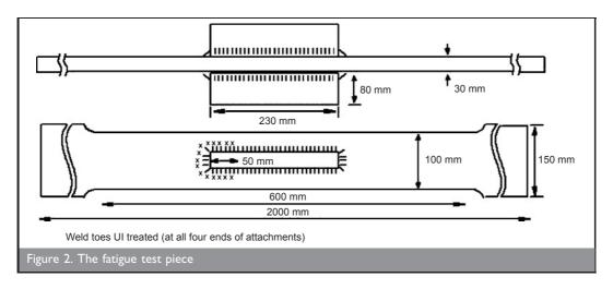
IP: 80.254.146.52 n: Mon, 20 Sep 2010 16:51:57 After pre-fatigue, the toes of the welds were UI treated to compensate for the damage and extend their remaining fatigue lives. All the treatments were made with the test pieces staying in the fatigue machines. The grooves produced by the UIT were inspected to confirm that the required profile had been achieved.
