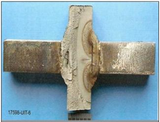
Figure 6. Fatigue crack from root and into main plate of a prefatigued and treated test piece.
